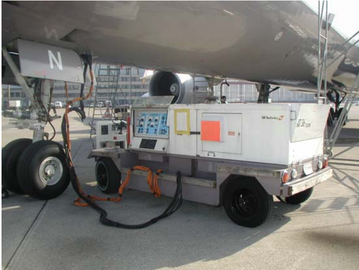
Figure 5-3: GPU for electrical power
